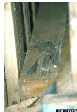
Figure 3. Asian longhorned beetle damage to boards and pallets. Photo courtesy of Larry R. Barber USDA-FS
