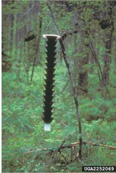
Figure 3. Lindgren funnel similar to those used to monitor for European woodwasp. Photo courtesy of Kenneth Gibson USDA-FS
