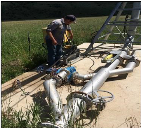
Figure 1: A mechanical hydropower system using irrigation water to drive a hydraulic pump. Photo: Blake Osborn
