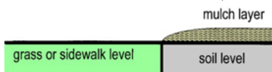
Figure 1. Mulch added above grade spills out onto the lawn or sidewalk.
