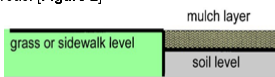
Figure 2. To keep mulch in place, drop the soil level in the mulch bed so the top of the mulch is at the grass or sidewalk level.
