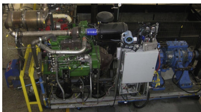
Fig. 2. 4.5 L 175 HP John Deere 4045 at the EECL.
