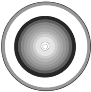
Example of a flicker checker showing smooth grey rings typical of electronic ballasts
