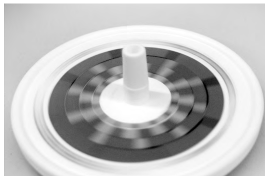
Flicker checking showing the checkered pattern typical of magnetic ballasts
