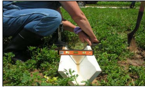
Figure 4: Placing Furrow Flume (notice a spirit level is used to ensure lengthways and crossways that the flume is flat).
