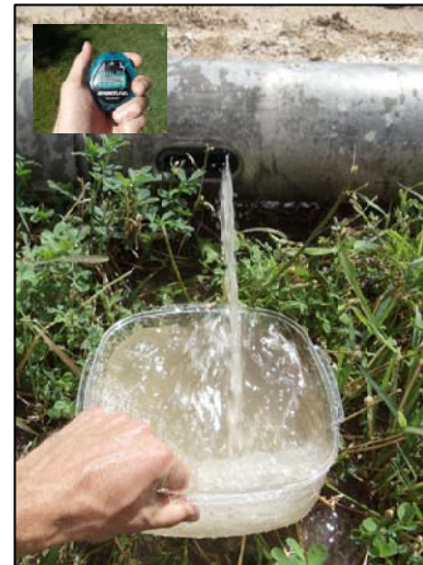
Figure 3 : A bucket test being timed for estimating furrow flow.
