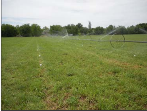
Figure 6: Catch-cans set in two rows next to the side roll. This side roll has a sprinkler throw of 40 ft. The innermost row is placed less than half of the throw (20ft) away from the side-roll and the second row is placed between half the throw distance and the outside of the Effective Irrigation Width or EIW (~35 feet away).
