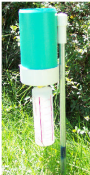
Figure 1: Irrigage built from thin-walled PVC pipe and plastic bottle
