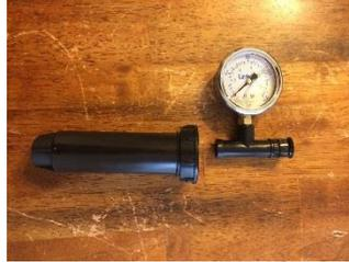
If you have rotor, impact, or rotator nozzles, use the pressure gauge below by placing the metal tip into the stream of water.
