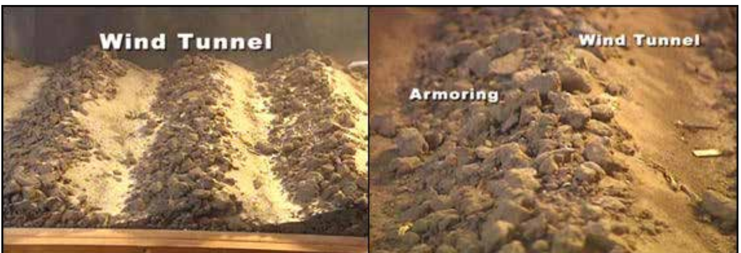
FIGURE 14. When a surface becomes armored wind erosion may temporarily be reduced.
