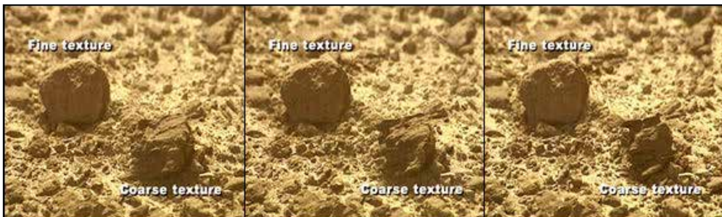
FIGURE 15. Time lapse photos of clod abrasion of fine vs. coarse textured soil, demonstrating faster erosion of the coarse textured clod.
