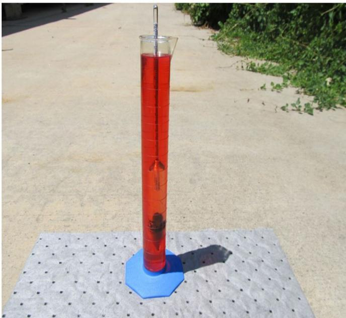
Figure 4. Hydrometer.
