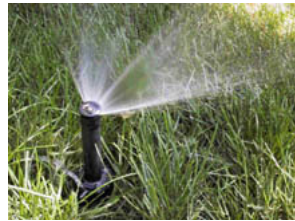
Figure 6: Pop-up spray heads produce a static spray band of a set pattern depending on the type chosen (1/4, 1/2, 3/4, full, or variable circle). Heads rise when water is turned on and retract when not in use.
