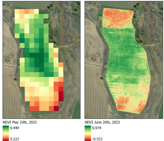
Left: Single field NDVI calculated from Landsat 9 imagery at 30 meter spatial resolution. Right: Drone based NDVI from a DJI Phantom 4 of the same field with 5 cm spatial resolution. Figure credits: Clara Mosso.
