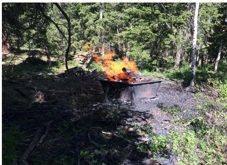
Figure 3. Metal biochar kiln processing feedstock.
