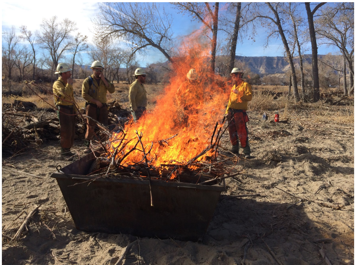
Figure 1. Metal biochar kiln processing feedstock in Utah.
