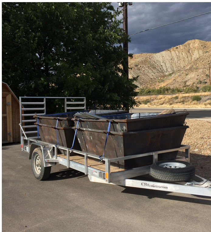
Figure 7. Flame cap biochar kilns stacked and ready for transport.
